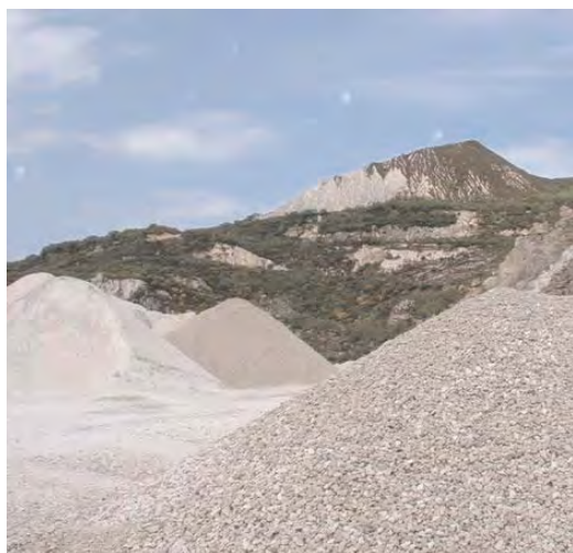
Figure 1. Photograph showing production stockpiles of china clay waste (foreground), uncrushed stent (mid-ground right) and an old spoil heap (background)
